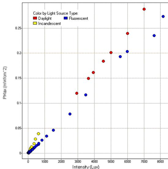
Figure 4: DSSC cells under different lighting conditions
