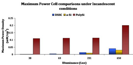
Figure 3: Cell comparison under incandescent lighting condition.
