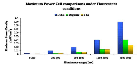
Figure 1: Cell comparison under fluorescent lighting condition.
