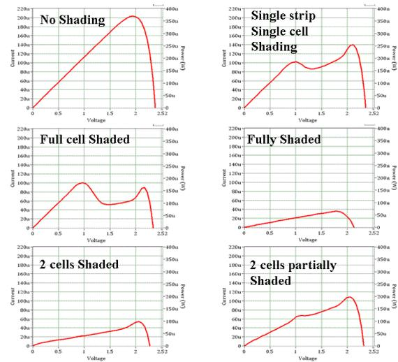
Figure 7: Effect of shading in a multi-cell topology.
