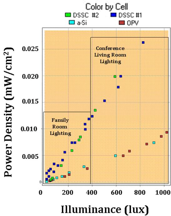
Figure 2: Windowing cell comparison for realistic indoor conditions.
